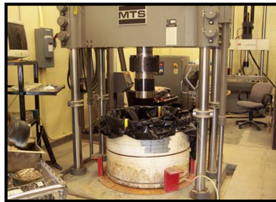
Figure 3.14 – Permanent Deformation Test on a Small Scale Specimen
